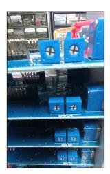
Test the HP/LF filters by activating the switch F.IN (down position).
